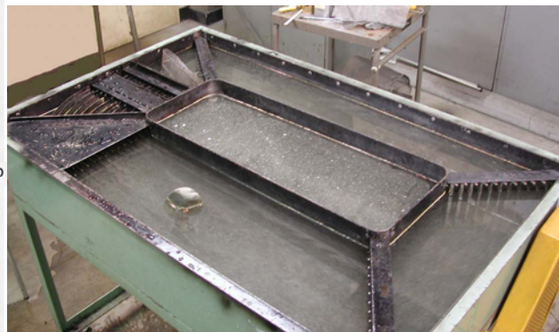
Fig. 10. Recirculation type water tank.
